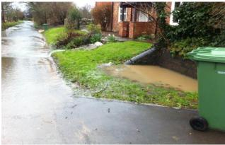
Flooding at the junction of New Barn lane and Eckington Road caused by the highway drain not being able to cope with the inundation and water forcing its way through the open grid in the adjacent field.
